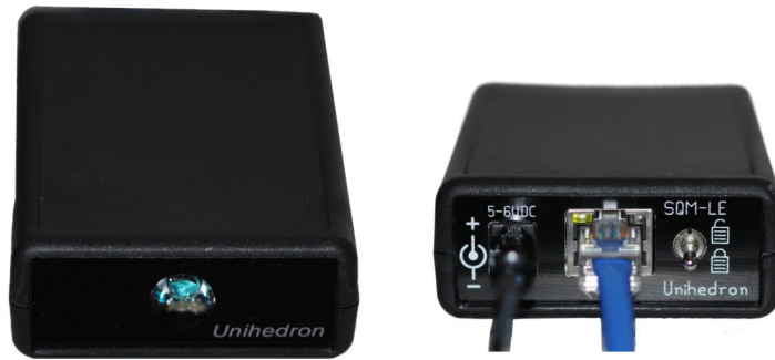
Fig. 3.— A unit of Sky Quality Meter - Lens Ethernet. The view in the left shows the blocking filter in light blue. The semi-conductor sensor is mounted under the filter. The view in the right shows (from left to right) the power and Ethernet inlets, and a switch for calibration purpose. (image source: Unihedron )
