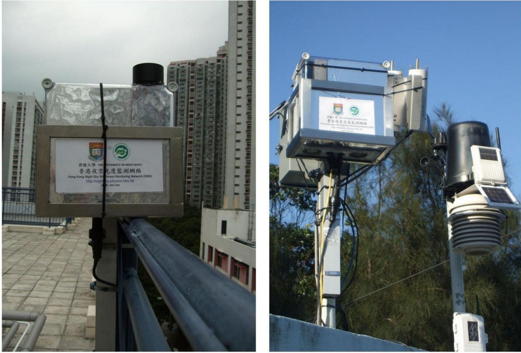
Fig. 4.— The WTS (urban, left) and iObs (rural, right) NSN monitoring stations. For the WTS station, a cylindrical light shield in black was applied to block direct lighting from nearby. For the iObs station, in addition to the night sky measurement module, two cloud sensors (narrow cylinders mounted on the right side of the rectangular box) were also mounted on the left-side pole, while an automatic weather station installed by the Hong Kong Space Museum on the right-side pole is also shown. Note that not all stations are equipped with cloud and weather observing equipments.
