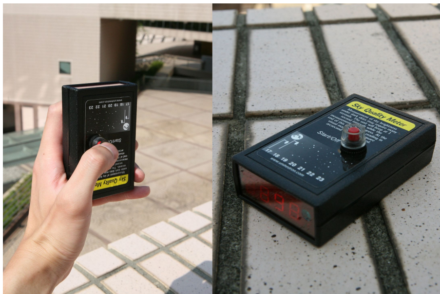
Fig. 4.— The Sky Quality Meter: the light sensor is located on the side of the near-infrared filter next to the display.
