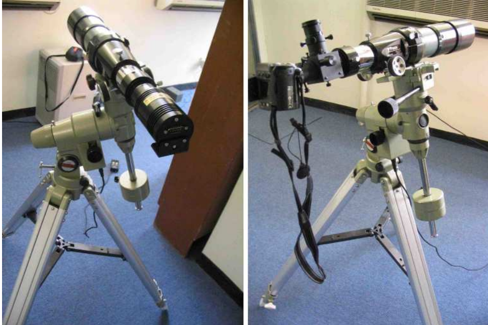
Figure 2: The whole setup. Left: Pronto with CCD. Right: Pronto with digital camera
